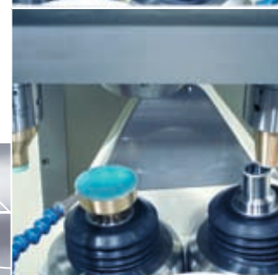
An integrated tool correction spindle system ensures fast and flawless adjustment of the polishing tool.
