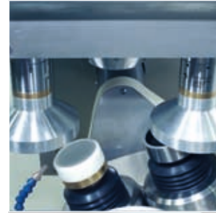
The S2/2 version allows for highest form accuracy, surface quality and process stability due to the use of 2 polishing spindles and 2 polishing agent cycles for rough- and high-quality polishing in one process cycle.
