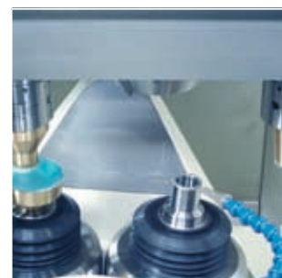
Deterministic aspheric polishing with the SCP 121 – zonal polishing with two tool spindles.
