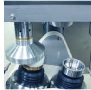
The SCP A 121, version S1/2, is capable of multistep polishing with individually controlled CNC parameters.
