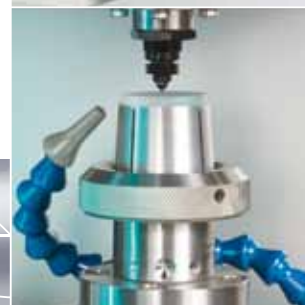
The center-thickness (CT) Control is an integral part of the comprehensive process control package.
