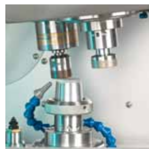
Rough and fine grinding of spheres using the double spindle technology.
