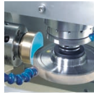
High stock removal and excellent contour accuracy is accomplished in the wheel grinding mode for aspheres.
