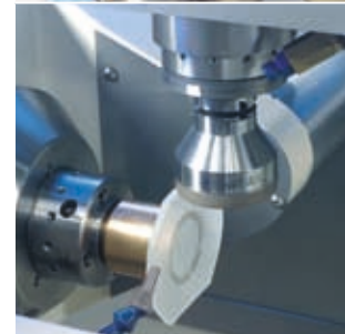
The list of processing options includes edging, centering, drilling, truncating and scooping as well as fabrication of prisms, flats and other special geometries.
