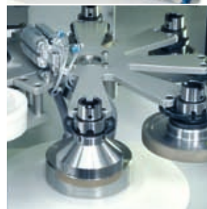
The automated tool changer allows an intelligent tool management including combinations of standard and form tools in one processing cycle.
