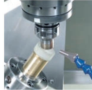
Cup wheel grinding of concave aspheres with standard tools.
