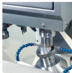
Rough and fine grinding of spheres using the double spindle technology (version S2/1).
