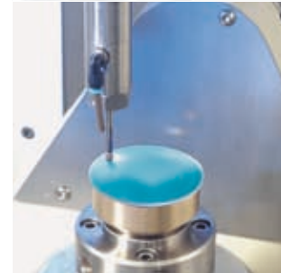
The in-process measuring technology (Contour Control) for the measurement of the aspherical lens contour and the automated correction calculation.
